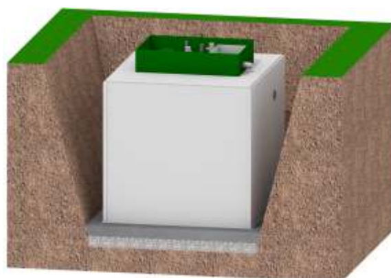
Instalace ČOV TOPAS S 15
